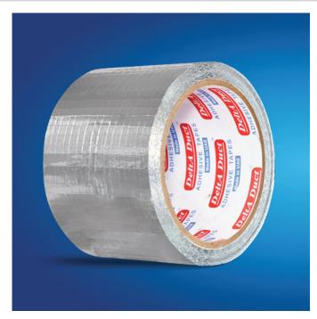
Foil-Scrim backing (Foil: 25u / 2-way Scrim: 5 x 5mm), combined with a transparent high performance solvent acrylic adhesive, protected by an easy-release silicone release paper.
