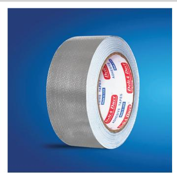
Delta Duct Alu Glass Tape is a foil-glass cloth backing (7u foil with a 10 x 10 mesh 85 gsm glass cloth) with strong high performance flame-retardant acrylic adhesive and protected by easy release liner.
