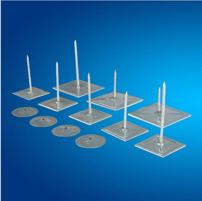
Delta Pins comprise of an aluminum nail (copper or steel alternatives on request) firmly mounted on a galvanized steel base which is backed by a self-adhesive, closed cell polyethylene foam substrate. Galvanized spring steel fastening clips (locking washers) are also supplied with the hangers available in different sizes, resistant to water, detergents, alcohols, aliphatic solvents and aromatic solvents.
