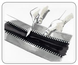
At a notch, cut a length equivalent to the perimeter required plus an overlap of 5 to 6 cm (2").
