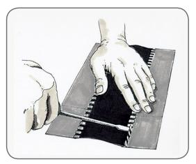
Lift the seam outwards at right angle.
