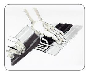
Coat the cloth with the appropriate adhesive, or pad. Join both sides and press together.
