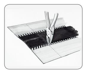
Make a cut at the edge of the seam section.
